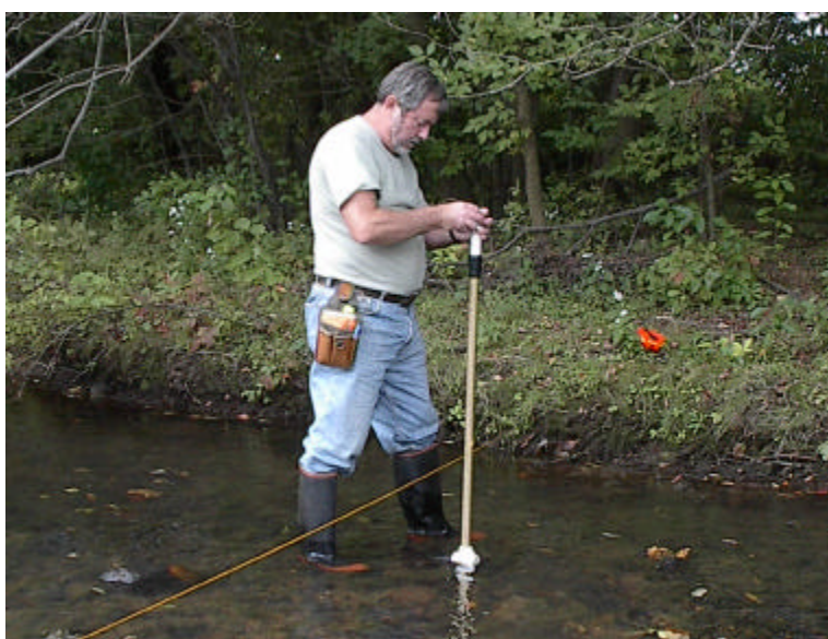
Figure 5.2 Collecting Stream Velocity and Water Depth Data
